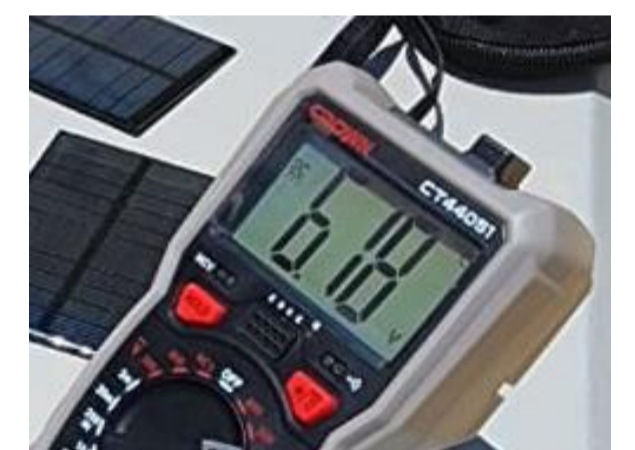
Solar Panels' voltage (max)
