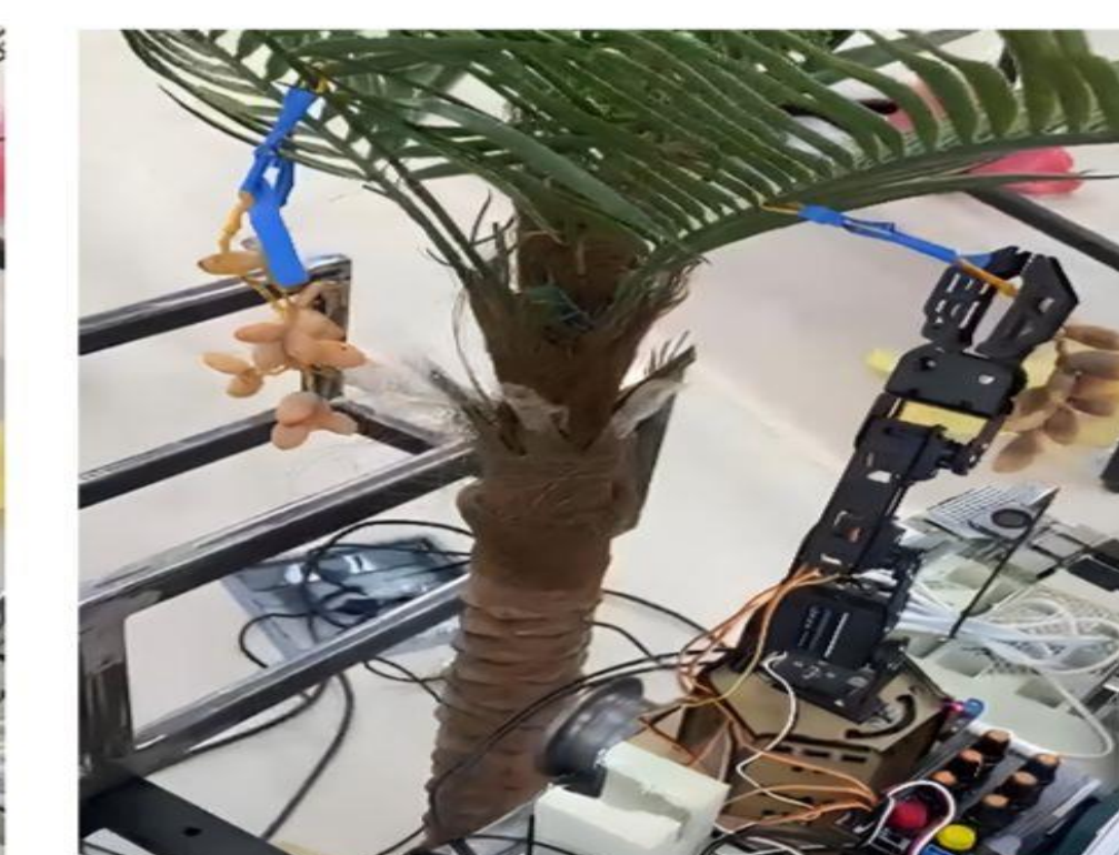
Step 4: Autonomous cutting Autonomous cutting is performed successfully.
