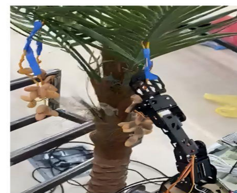
Step 3: Grasping End-effector grasps the date bunch.
