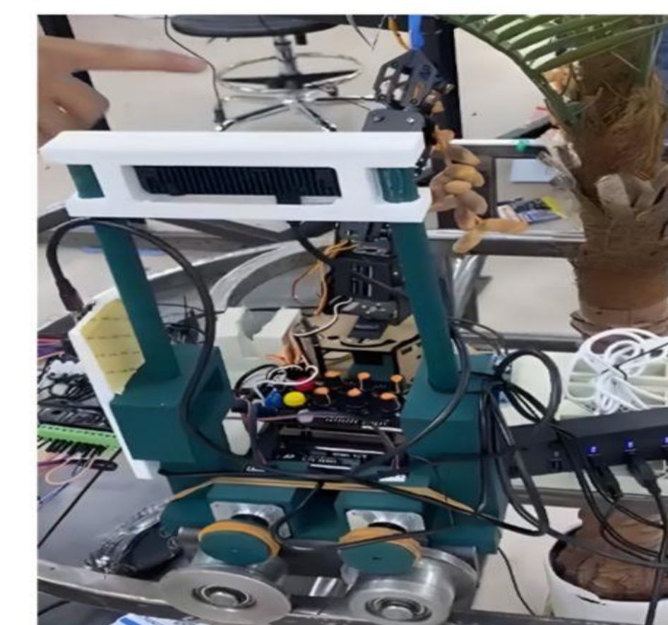
Step 1: Detection Robot detects bunch then rail stops automatically.
